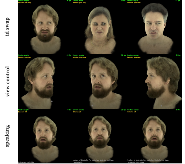
Fig. 8. STEER deployed in a real-time setting at 25 fps. Row 1 ( id swap ): same pose driving three different identities through UHAP. Row 2 ( view control ): free-viewpoint rendering of the same identity. Row 3 ( speaking ): live audio-driven speaking with semantic-control overlays (emotion, behavior).
